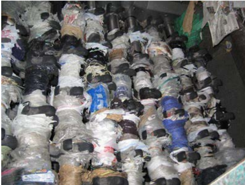
Film Plastic Tangled in Processing Equipment
